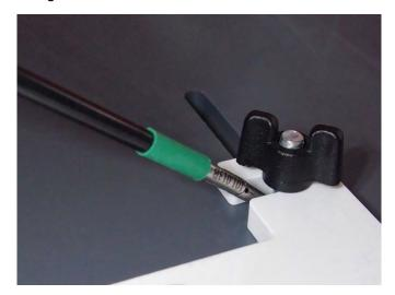
**Time measuring** starts/stops at the moment when both instruments have entered/left the operating field.
