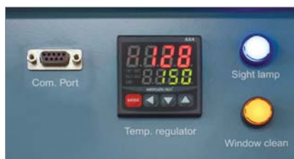
Electronic over temperature shutdown system.
