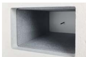
1100°C model (4-side molding type heater)
