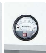
Differential pressure gauge
