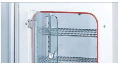
Sealed glass door for contamination prevention.
