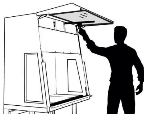
Cleaning the front window
